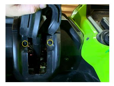
• Replace the bottom half of the steering column rubber boot
