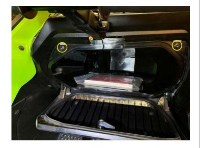
• Install the bottom steering wheel cover
