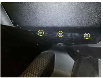
• Install one push pin in the back of the glove box
