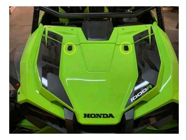
Remove four 10mm bolts, four push pins and five 5mm allen bolts to remove top of dash
