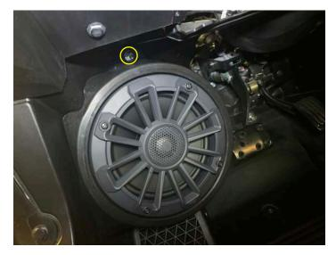
• Tighten the 5/16" bolt in the fender area
