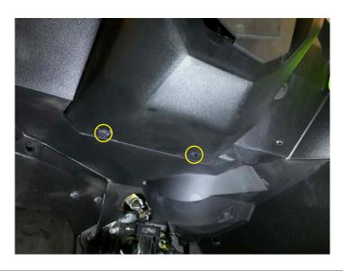
• Remove the bottom steering wheel cover
