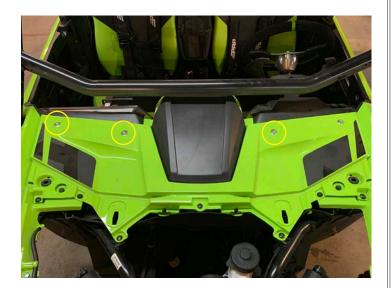
• Install hood by turning two latches
