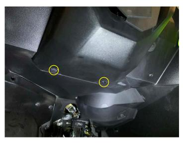
• Install the two push pins behind the rubber boot
