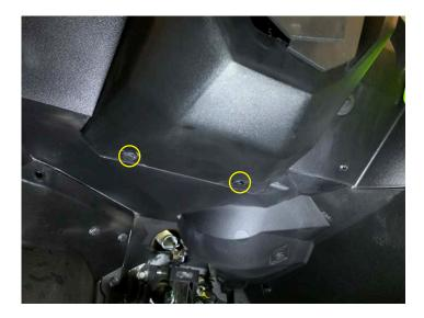
• Install the two push pins behind the rubber boot
