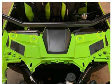
• Install hood by turning two latches
