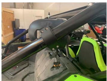
Adjust the alignment by loosening the M6 bolt as shown to swivel the speaker (When in the position you want then tighten the bolt)
