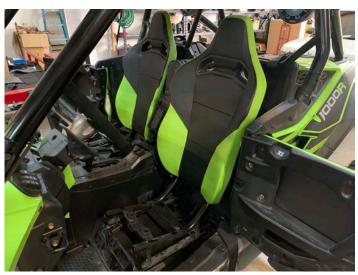
Slide driver seat forward and install two 12mm bolts on rear of seat
