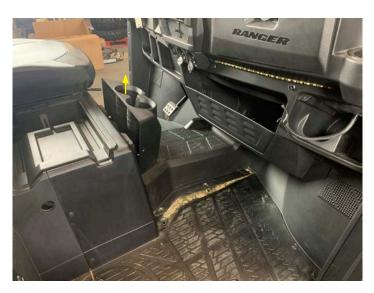
Using a small flat head screwdriver, push in the center and remove the six clips on the passenger side
