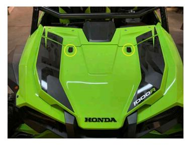
Remove four 10mm bolts, four push pins, and five 5mm allen bolts to remove top of dash
