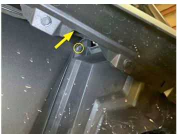
• Remove three push pins from inner lip of fender
