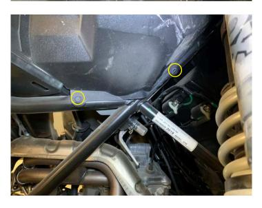
Install the air intake cover from the passenger rear fender area by installing ten push pins (Each location to follow)
