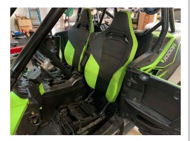
Remove two push pins on front of passenger seat and then remove the covers
