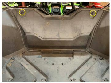
Install one 5 mm allen bolt and one push pin from passenger kick area
