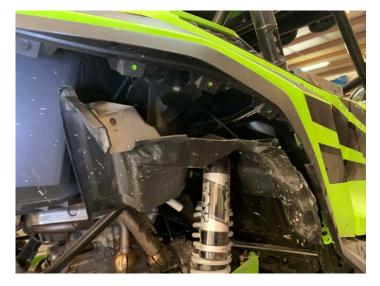
• Install two push pins behind the passenger rear shock
