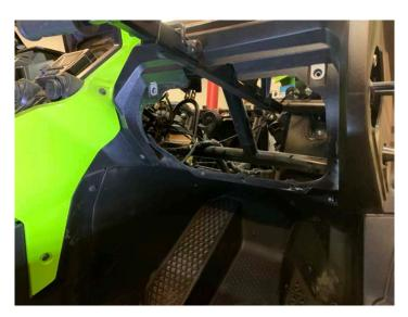
Remove one 5 mm allen bolt and one push pin from passenger kick area
