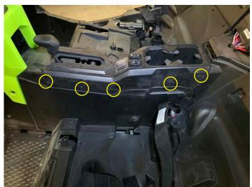
Using a small flat head screwdriver push in the center and install the six clips on the passenger side
