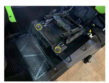
Release latch at front of driver and passanger lower cushions to install
