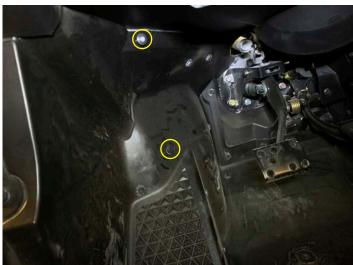
• Install the bottom steering wheel cover
