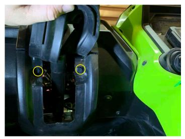
• Lift up the bottom half of the steering column rubber boot
