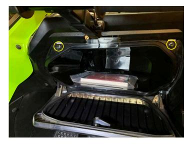
Install one 5mm allen bolt and one push pin from the drivers kick area
