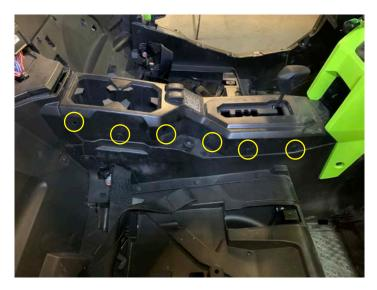
Remove the five push pins on the driver side console like on the passenger side
