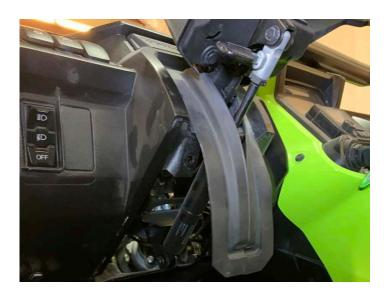
• Install the two push pins on the bottom of steering column cover
