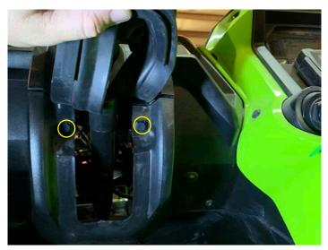
• Remove the two push pins on the bottom of steering column cover
