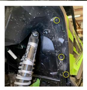
• Remove two push pins from outer fender
