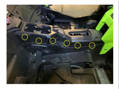
Drop center console downward starting at cupholder and install in vehicle
