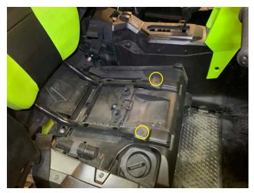
Remove two 12mm bolts and two 12mm nuts on the passenger seat base
