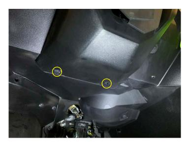
• Remove the bottom steering wheel cover
