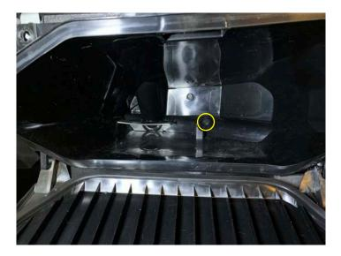
• Remove three push pins from below the glove box
