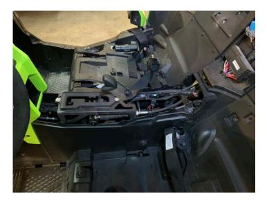
Install the five push pins on the driver side console like on the passenger side
