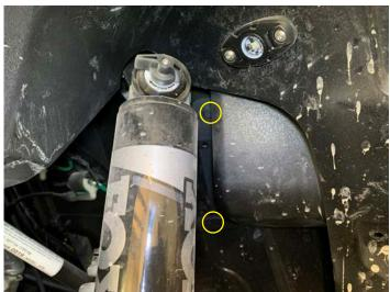
• Install two push pins from outer fender
