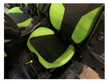
Remove two 12mm bolts on front of drivers seat
