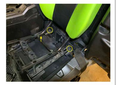
Install two 12mm bolts on front of drivers seat
