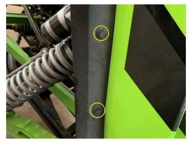
• Remove two push pins behind the passenger rear shock
