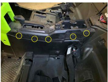
Place gear selector to "H" and remove the top of the center console
