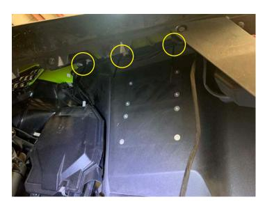
• Drill ½" hole on either side of the bed area as shown
