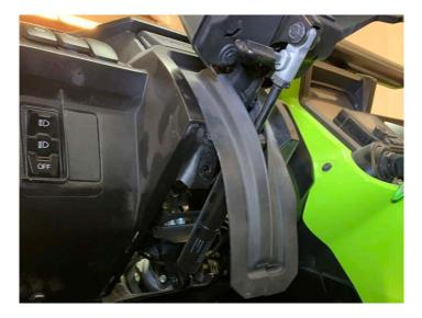
Remove one 5mm allen bolt and one push pin from the drivers kick area
