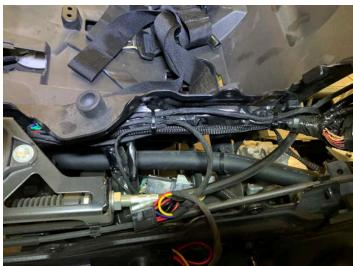
Pass the wires through the rear firewall and upward between airbox and firewall
