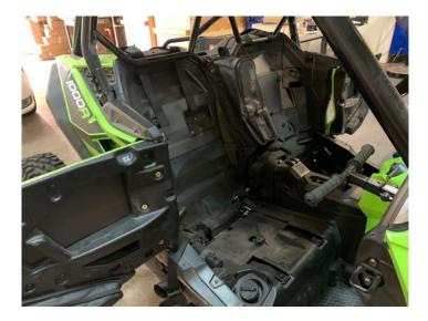
Pull top fuse access panel toward front of vehicle and remove
