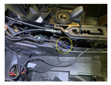
• Zip tie wires in center console along the OEM harness
