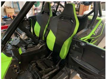
Slide driver seat forward and install two 12mm bolts on rear of seat
