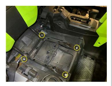
Install two push pins on front of passenger seat and then remove the covers
