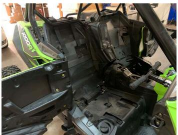
Install two 12mm bolts and two 12mm nuts on the passenger seat base
