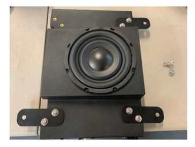
Place subwoofer enclosure under driver seat area and pass the harness through small opening pictured and pull toward top of center console
