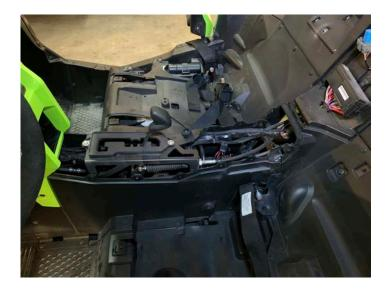
Install the five push pins on the driver side console like you did on the passenger side
