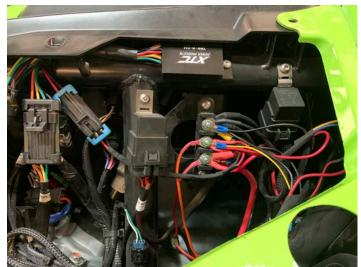
Plug RCA into the NA2-400.2 and run to the front RCA outputs of the radio
