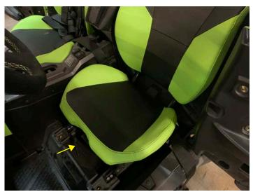
• Install half mud guard with 6 push pins
