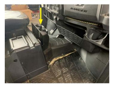
• Insert four push pins on passenger side console
