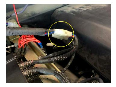
Connect the subwoofer extension harness to the NA2-400.1 amplifier harness
