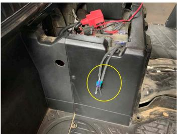
Drill 1.25" hole and pass subwoofer connection through hole and place grommet
